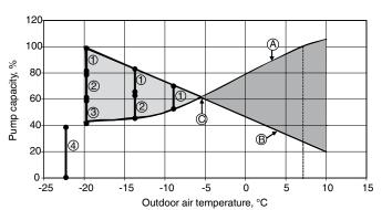
Operating range, in which the heat pump capacity is lower than the building thermal load
