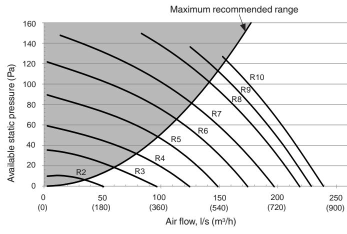
Pressure drop (Pa) for supply and return air plenum boxes as a function of the number of spigots ( $\varnothing 200 \text{ mm}$ )
