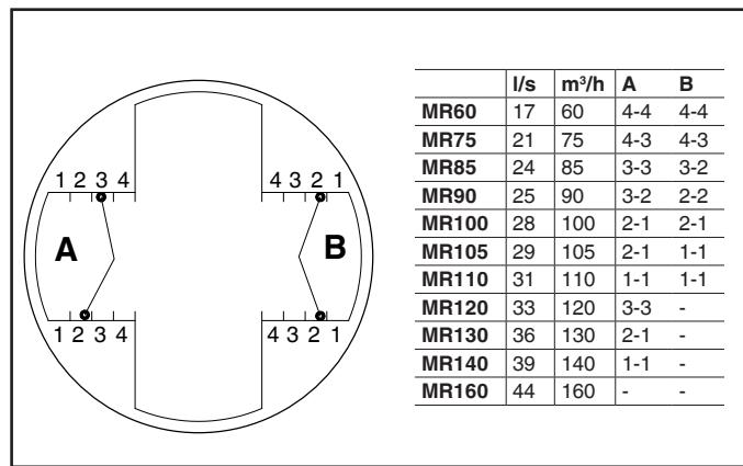
The 17 l/s (60 m<sup>3</sup>/h) or fresh air controller may be modified on site by relocating or removing two plastic restrictors in order to increase the maximum constant fresh air flow capacity to 44 l/s (160 m<sup>3</sup>/h).
