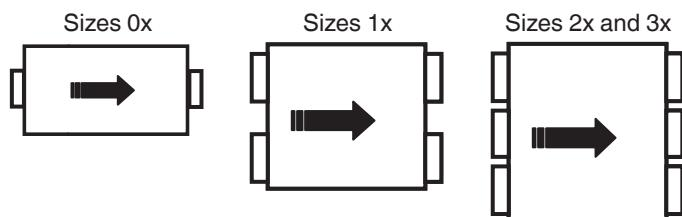
This version does not allow the use of 200 mm diameter spigots on the sides. Filter removal is from below.
