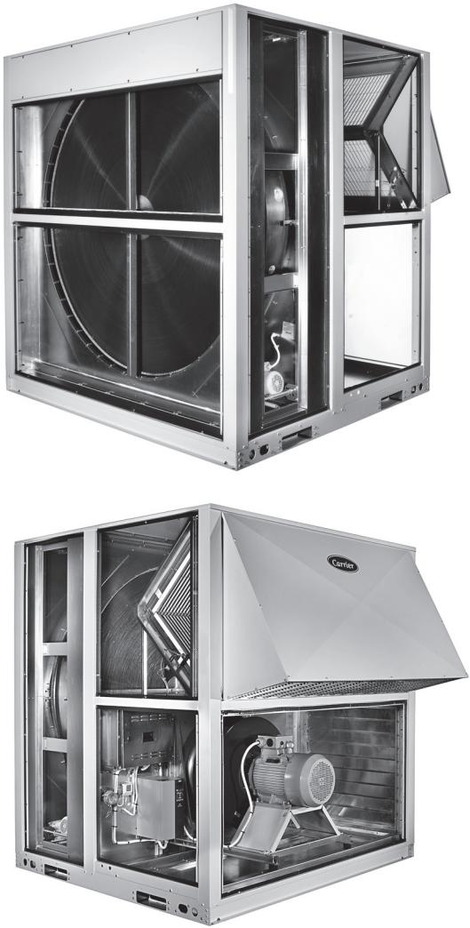
The ERM is an individual dual-flow unit, equipped with a high-efficiency Eurovent-certified air-to-air heat recovery wheel with 63% to 88% efficiency, an integrated variable-air-volume plug fan and a control system for plug-and-play installation. The modules are specially designed to ensure economical indoor air extraction and to take in fresh air to meet current and future requirements for high-energy-efficiency buildings.
